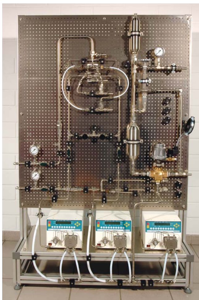
Exhibit 6.1 Nitroglycerine production plant (>100 l/h solution) using microstructured reactors set in operation in Xi'an, China (courtesy IMM, Germany)
