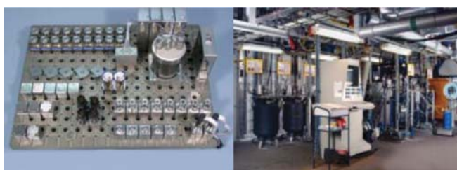
Exhibit 5.1 Ehrfeld modular microreaction toolbox and pilot/production plant system
